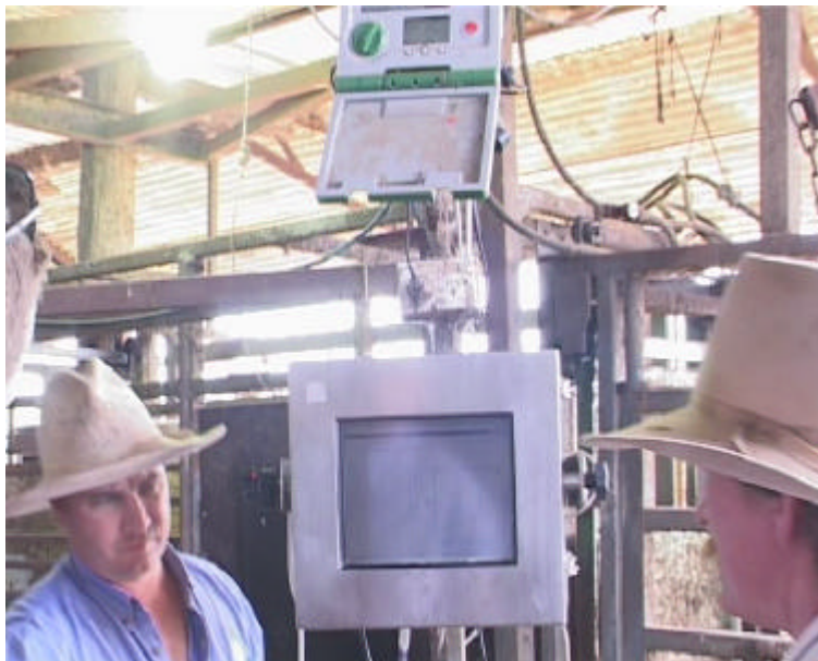
Figure 6 - Collection of Induction Data using Industrial PC
